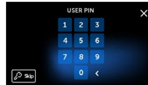
To finish the batch approval for use, user must tap **CONFIRM** button, and enter personal PIN code (tap **Skip** to bypass this step). Then, Hello screen is displayed and the autoclave is ready for the next process.
