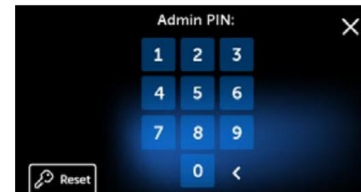
Before activating user identification, 4-digit admin PIN must be set (default admin PIN is set to 0000). The admin user is requested to enter PIN each time any changes are done. If the PIN is lost, the user can use **Reset** button in the lower left corner.
