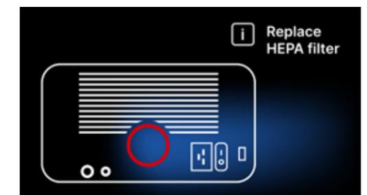
During regular operation, info screens concerning replacement of individual elements or required service inspection are displayed alternately. Counter values displayed in yellow or red do not prevent the device from operation. However, exceeding the required inspection date may significantly affect the device's operation and the load sterilization process.
