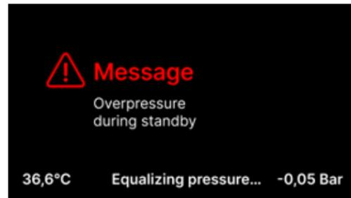
Screen about overpressure or underpressure resulting from the natural processes of cooling the chamber. It can occur immediately after starting the machine.
