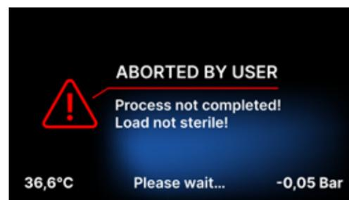
You can freely open the device now. The following screen will be displayed when the chamber is opened. By selecting the **RESTART** field, you can return to the start screen.
