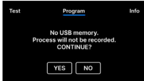
If the USB drive has not been inserted in the device, the USB symbol is **not** displayed in the bottom right corner of the screen, and a message about the missing USB drive is displayed. The program data will not be saved. You can continue working without saving the data on the USB drive by pressing the **YES** field or stop working by selecting the **NO** field to insert the drive in the port and start the program from the beginning.
