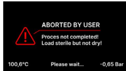
Message resulting from interruption of the process after the sterilization stage - during drying.
