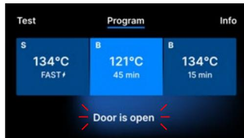
When the chamber is opened, the **DOOR OPEN** symbol blinks.
