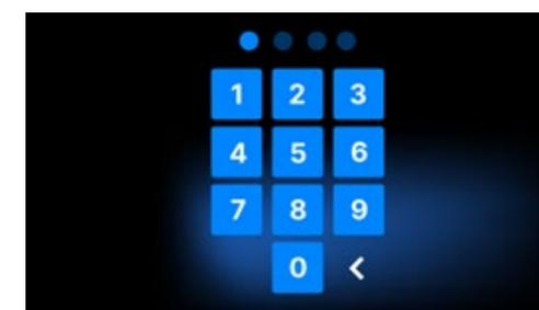
If the code is entered incorrectly, a message will be displayed on the screen. Enter the code again. The arrow enables cancelling incorrectly entered digits. When the code is entered correctly, the start screen will be displayed.
