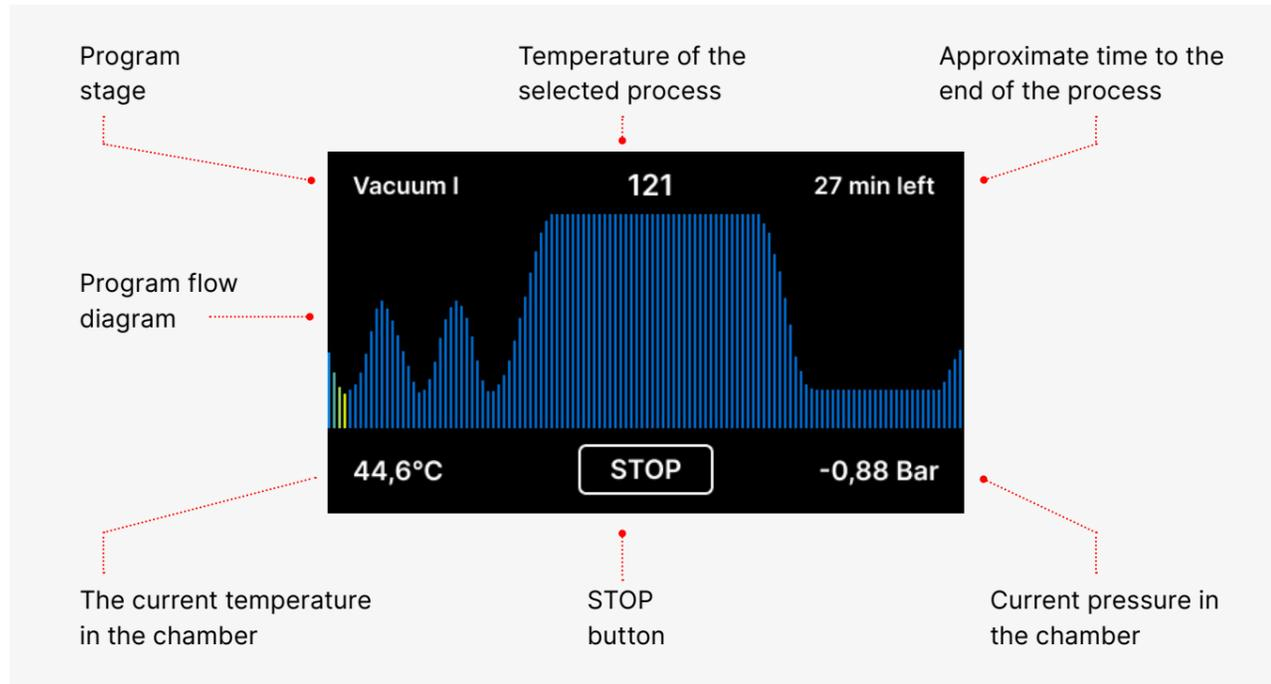
When a program is being run, the screen displays the temperature of the selected sterilization program **121°C** or **134°C**, the current temperature of the process chamber in the bottom left corner **44,6°C**, the pressure currently in the chamber in the bottom right corner **-0.88 Bar**, while the process duration left is displayed in the upper right corner of the screen **25 min left**. This is the expected time, which may be extended due to the mass and type of charge.
