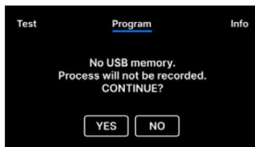
If the USB drive has not been inserted in the device, the USB symbol is not displayed in the bottom right corner of the screen, and a message about the missing USB drive is displayed. The test program data will not be saved. You can continue working without saving the data on the USB drive by pressing the **YES** field or stop working by selecting the **NO** field to insert the drive in the port and start the test program from the beginning.
