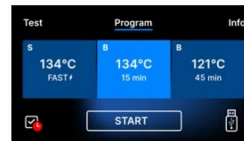
Red mark on the icon reminds the user about closing the doors before leaving. Auto test will not start when door are open.
