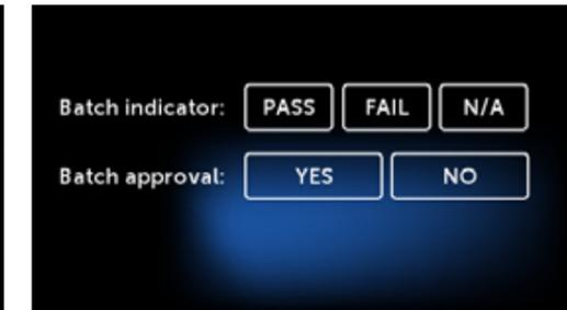
After the process is completed successfully, the screen with approval options appear. Open the drawer and make visual assessment of the load.
