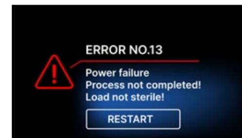
If the restart is forced by process error, before returning to the start screen, you must enter the 4-digit security code **0000**.
