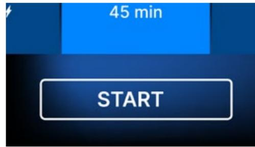
When the chamber is locked by turning the lock knob clockwise, the display will show the **START** symbol, indicating the chamber has been closed correctly. Now you can select the program by pressing the symbol of the temperature you want to perform the sterilization for example in 121°C or 134°C. The selected program is initiated by pressing the corresponding **START** symbol.
