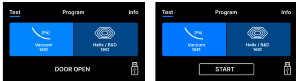
By pressing the **Test** field, you can go to the test program menu. From here you can select the vacuum leak test program and the Helix/B&D test program. Select the appropriate program by pressing the relevant field on the display. When the process chamber is closed, the **DOOR OPEN** information changes to **START** and by pressing this field you launch the selected test program.
