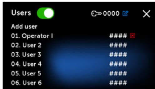
The new user with the PIN is added. You can delete the user by tapping red cross to the right of the PIN. Admin PIN can be changed from this screen, by tapping the small key icon at the top of the screen.
