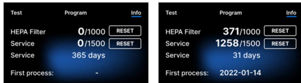
The number of performed processes is on the left and on the right side – the number at which the given element should be replaced or a service inspection performed. After replacing a filter, the values can be reset by the user by pressing the button. The service inspection value can only be reset by an authorised service.
