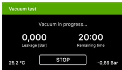
When the vacuum leak test program is selected and launched with the **START** button, the vacuum leak test progress screen is displayed. Information on pressure loss in the process chamber, and the test duration are displayed.
