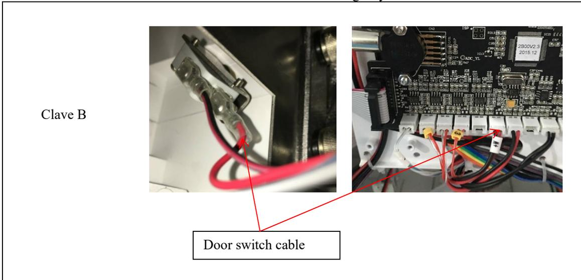
Case 1: The door switch cable is disconnected. Check the connector on the mainboard and the switch.
