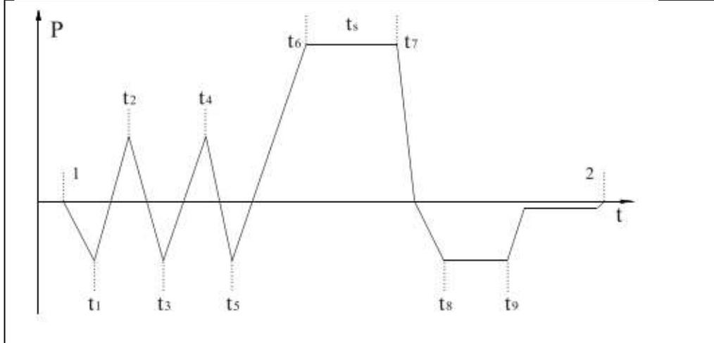
Alarm condition: At the rising pressure phase, it takes excessive time to reach the next status. From t1 to t2, t3 to t4, t5 to t6
