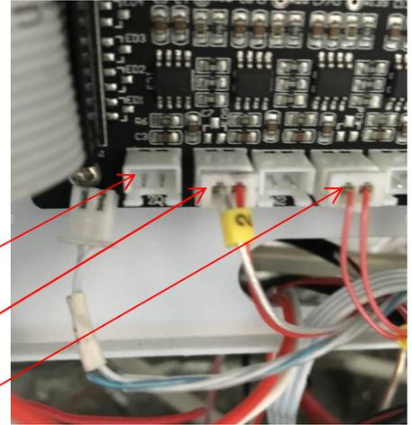
Case 1. The sensor cable is disconnected, or the sensor doesn't work.
