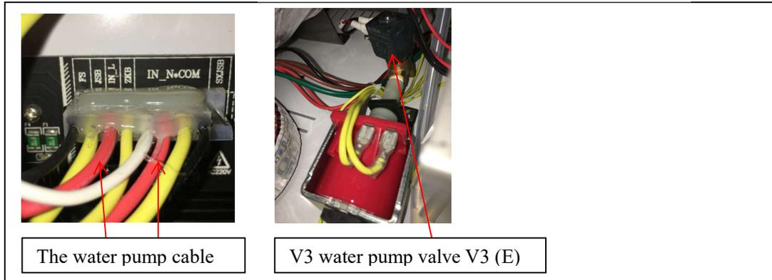
Case 3: The temperature is higher than 100°C and there is water inside the chamber when E24 appears. There is a leak somewhere.
