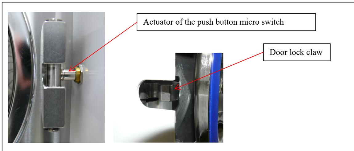
2.2 The door slide does not connect well with the door close switch. Adjust the lever of the micro switch; bend the lever to make the door slide connect well after the door is closed (for model C).
