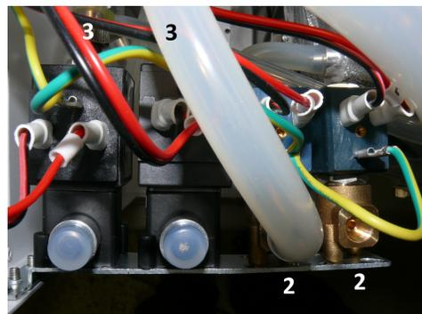
The coil voltage is 24V DC, and the resistance of the coil is about 60Ω.
