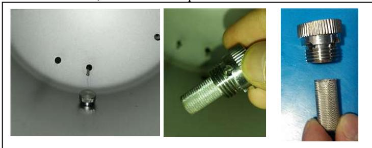
Case 3: The water release valve is blocked or does not work.
